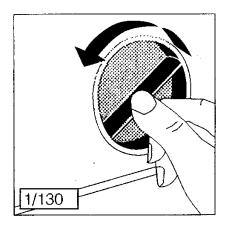
Remove foreign bodies from the pump housing. Always also check by hand that the pump impeller runs freely.
